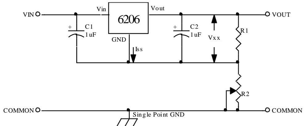
$$V_{out} = V_{xx}(1 + R_2/R_1) + I_{ss}R_2$$
