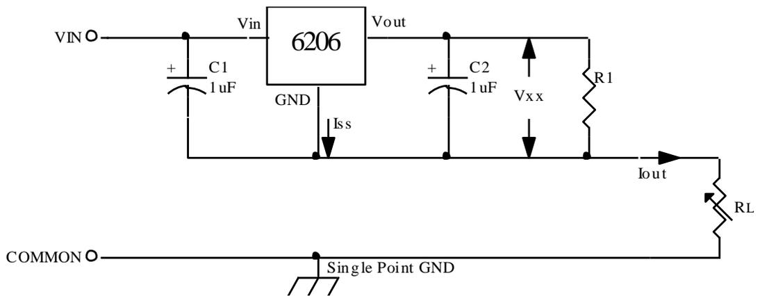
$$I_{out} = V_{xx} / R_A + I_{ss}$$
