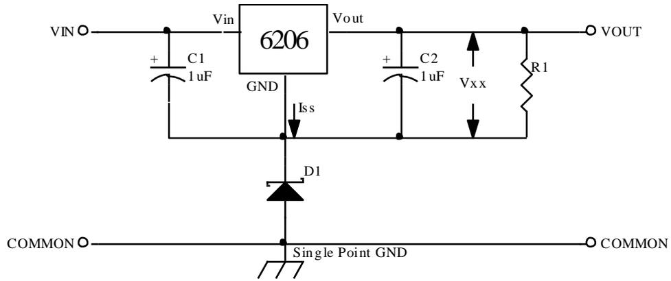
$$V_{out} = V_{xx} + V_{D1}$$
